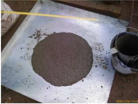
High slump SCC concrete ensures total fill and zero voids
